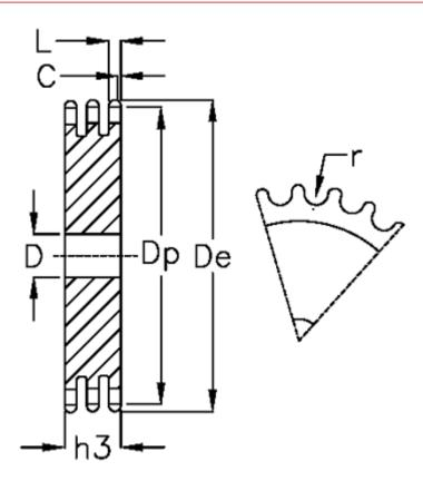
С = 2 D = 25 De = 203.3= 194.35Dp For chain size =  $3/4 \times 7/16$ For chain type = 12 B-3 = 49.8
